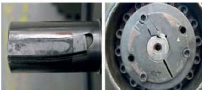
Figure 4: Damaged Key Due to Torque Transients
