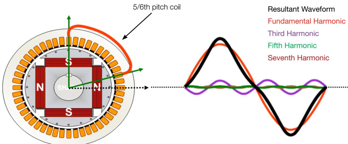
Figure 2: Short 5/6th pitch winding machine with resultant waveform of the output phase voltage
