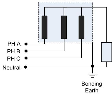
Figure 4c: Star point connection via impedance (restricted fault current)
