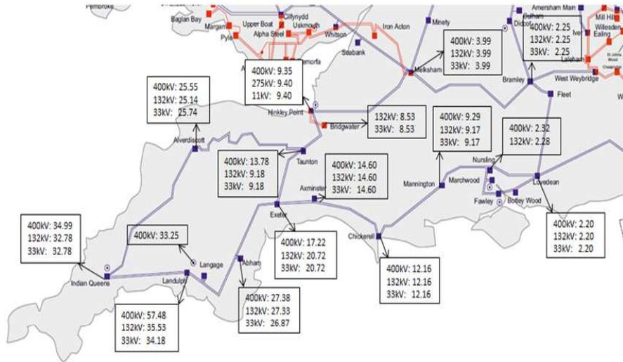
Figure 3 Change in Voltage angle Across the Transmission system
